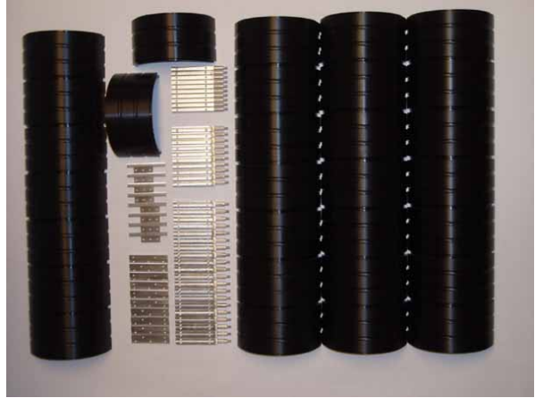
Tires, rims (made of aluminium and than plated with nickel), holders for the mudguards and the mudguards (everything is handmade)
